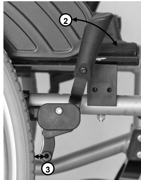
Brake disengaged (wheelchair rolls)
