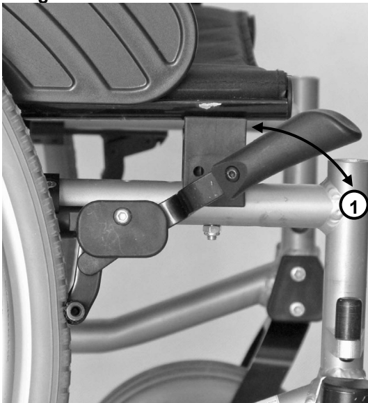
Brake engaged (wheelchair doesn't roll)
