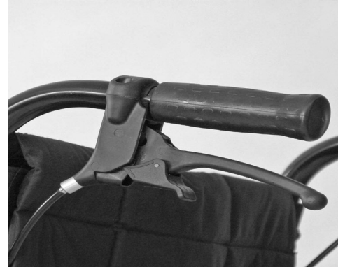
Brake engaged & locked
